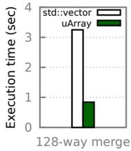
Figure 11: On-demand growth of uArrays vs. std::vector
