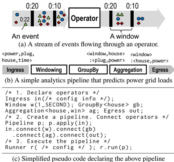
Figure 2: Example stream data, operators, and a pipeline
